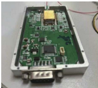
(a) F-P微腔自注入锁定窄线宽激光器模块 (a) F-P micro-cavity self-injection locked narrow-linewidth laser module
